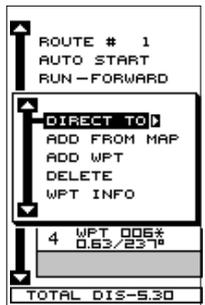
Now highlight the first waypoint in the route that you wish to start with and press the right arrow key. (The first waypoint in the route is used in this example.) The screen shown above right appears. Now select "DIRECT TO" and press the right arrow key.
