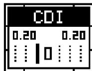
The CDI's range shows beneath the CDI label. On the above screen, the CDI range is .20 mile, which is the default. You can adjust the range by selecting the "ALARMS/CDI" label on the main menu. This is also shown by the dotted lines at the far left and right side of the CDI. If the solid line is on either of the dotted lines, then you are 0.20 mile off course. Remember, if the line moves to the left, then you are too far to the right of the desired course line and vice-versa.
