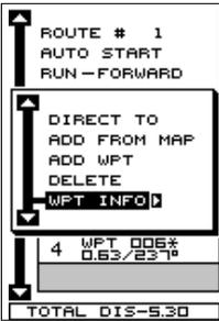
The selected waypoint number appears at the top of this screen. Information about the waypoint shows at the bottom of the screen. When you're finished with this screen, press the EXIT key to erase it.
