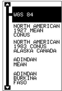
The WGS-84 label is highlighted. To change it, simply press the up or down arrow keys to highlight the desired datum, then press the ENT key. This selects the datum and erases the select datum menu. To erase the menu without changing the datum, simply press the EXIT key.
