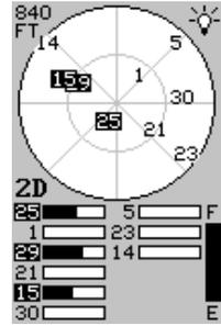
A battery level indicator on the lower right side of the screen shows approximately how much life is in the batteries. This runs from "F" (fully charged) to "E" (expired).
