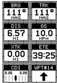
This screen is composed of eight digital boxes. Track (TRK) and ground speed (GS) data are all that show if you're not navigating to a waypoint. If you are navigat-
