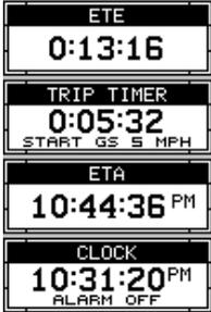
The trip timer measures the total time you have been travelling. It starts counting when you exceed a preset speed. The default is 5 miles per hour. You can adjust this time from zero to 200 m.p.h.. To do this, press the MENU key, then select "TRIP TIMER SETUP" menu. The screen at right appears. Highlight the "START GS" label, then press the left or right arrow keys until the desired speed appears. Press the EXIT key to erase this screen.
