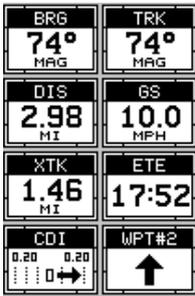
the present position. Therefore, the unit shows navigation information to waypoint number 2. The first leg of the route, from #4 to #2 is shown on the screen by a dotted line. Once you arrive at waypoint number 2, the unit switches to the next waypoint in the route, and so on. The rest of the route navigation is used normally.
