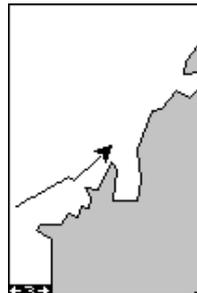
Using the map is as simple as pressing the PAGES key, then highlighting “MAP 1”. A screen similar to the one at right appears. The arrow flashing in the center of the screen is your present position. It points in the direction you’re travelling. The solid line extending from the arrow is your plot trail, or path you’ve taken. The plotter’s range shows in the lower left corner of the screen. In this example, the plotter’s range is two miles from the left edge of the screen to the right.
