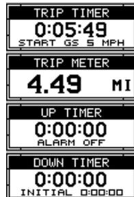
The up timer starts at zero and counts up. The up timer also has an alarm. The down timer starts from a user setting and counts down to zero.
