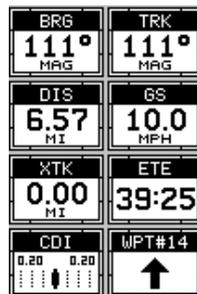
The destination arrow shows the direction to the destination when the top of the screen is pointing in your direction of travel.
