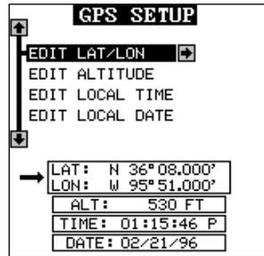
This is the GPS initialization screen. The position, altitude, time, and date the AccuMap Sport is currently using to find the satellites is shown at the bottom of this screen. Changing these values to your local position and time will speed the position lock.
