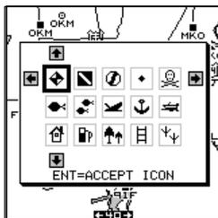
Press the arrow keys to move the black box to the desired icon, then press the ENT key to assign it to your waypoint. The unit returns to the waypoint screen with the icon you selected assigned to the waypoint.
