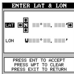
back to the number you need to change, and change it. If you want to change the entire latitude number, press the WPT key to erase it and start over. To exit completely out of this screen without saving the position, press the EXIT key.
