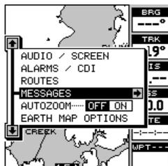
When you're finished with this screen, press the EXIT key to return to a mapping, navigation, or windows screen.
