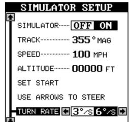
To turn the simulator off, press the MENU key, then move the black box to the "Simulator Setup" label. Finally, press the left arrow key.
