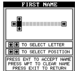
This is the first name entry screen. Press the up or down arrow keys until the first letter appears that you want to use. When it does, then press the right arrow key to move to the next letter. Continue this process until the I.D. is complete. You can press the WPT key to completely erase all of the characters you entered and start over, if you need to. Pressing the EXIT key erases this screen without accepting any input. When the first name is correct, press the ENT key.
