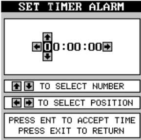
To start the timer, press the MENU key, then move the black box to the "Dn Timer STOP/GO" label. Press the right arrow key to start the timer. The timer continues counting until you stop it. If you turn the up timer's alarm on (press the right arrow key when the black box is on the (Up ALM...Off/On label), it will sound a tone when it reaches the time you entered in the up timer set menu. Press the EXIT key to silence the alarm.
