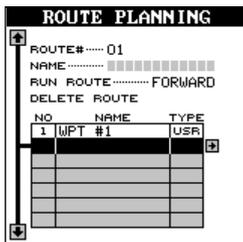
Move the cursor (using the arrow keys) until it's on the exact location that you want to add to the route list. When it's there, press the ENT key.
