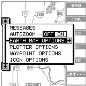
Using the arrow keys moves the black box to highlight different menus on the list. Pressing the right arrow key selects the menu.
