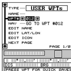
When the desired waypoint number is showing, press the down arrow key to move the black box to the "EDIT LAT/LON" label, then press the right arrow key. The screen shown at right appears. To enter the latitude, simply move the black box using the right and left arrow keys, then press the up or down arrow keys until the desired number appears. If you make a mistake, simply move the black box
