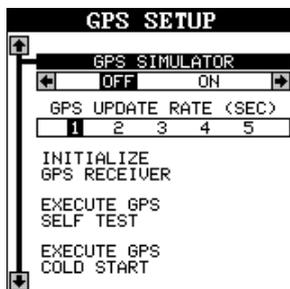
Using the down arrow key, highlight the “Initialize GPS Receiver” menu, then press the right arrow key. The screen shown at right appears.
