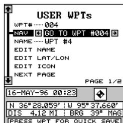
In this example, we recalled waypoint number 4. It's 4.12 miles away from our present position on a bearing of 39° magnetic, which is roughly north-northeast.
