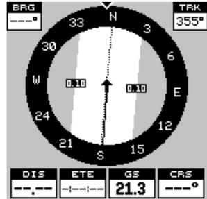
Your speed over ground or Ground Speed is shown at the bottom of this screen. In this example, the ground speed is 21.3 miles per hour. The screen looks like this when you're not navigating to a waypoint. (See page 30 for information on waypoint navigation.) If you navigate to a waypoint, the screen looks like the one at right and below.
