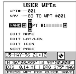
Press the up or down arrow keys to select the first letter in the name. Press the right arrow key to move the black box to the next position in the name. Repeat this sequence until you've entered all of the letters in the waypoint name. Press the ENT key to accept this name, the WPT key to erase all characters in the name, or the EXIT key to leave this screen without saving any changes.
