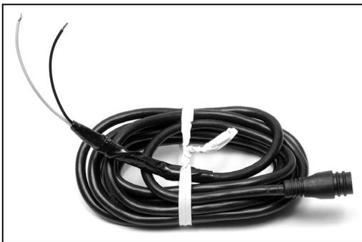
**Strip the ends of the VHF radio's data wires. Connect them to the pre-stripped wires of the Cuda 240i's data cable (shown right).**
